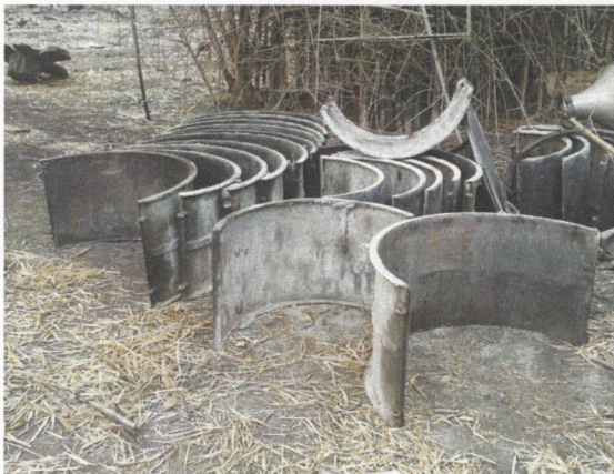
Concrete ring molds
