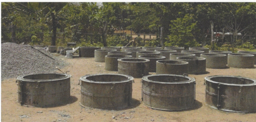
In process and completed rings for building wells and latrines
